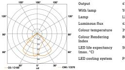
47 W Yes, STEINEL LED system LED cannot be replaced 4367 lm 3900 K 80-89
