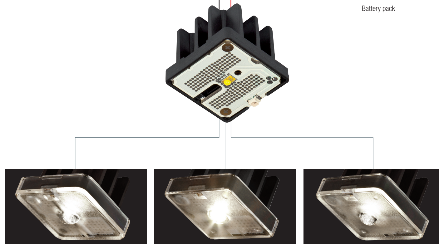
Lungaluce Lens installed at 3m height covers an escape route of 11,8m granting 1 lux in the middle and >0,5 within 1m
